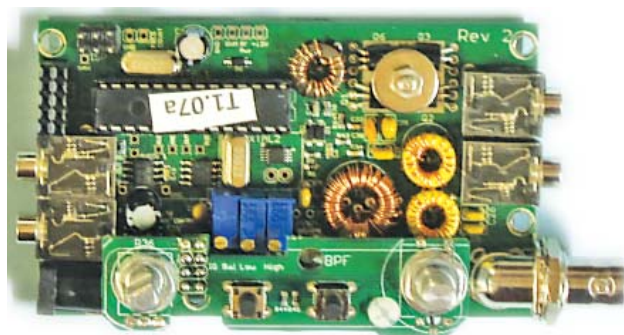
Figure 1 — The main circuit board carries most of the components for the receiver and transmitter sections. The microcontroller (white label) is at the upper left. T1 is the larger toroid near the center, and the socket that connects to the display board is in the upper left. The driver and final amplifier transistors are at the upper right, under the washer.
