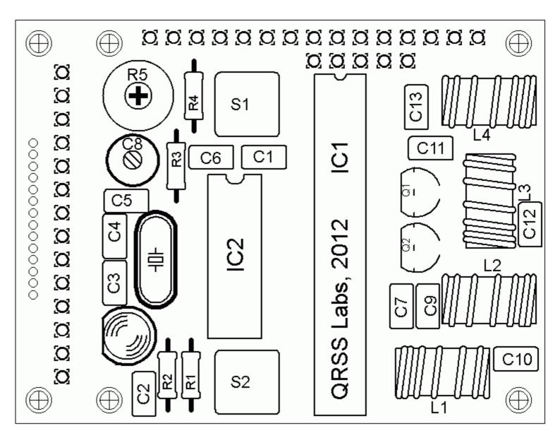
Pay special attention to the orientation of the semiconductors. For IC1 and IC2, the dimple in the PCB silkscreen must be aligned with the dimple at the top of the IC socket and the IC. The LED image on the PCB shows a flat along one side, which should be aligned with the flat on the LED. Similarly, the transistor.
