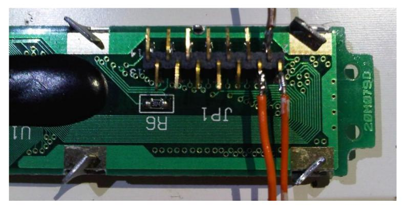
Another alternative LCD mounting option is to insert the LCD into the PCB in the normal way, but before soldering the pins, bend the pins gently 90-degrees, then solder. This method puts the LCD at right-angles to the PCB and is very nice for front-panel mounting; note, however, that the PCB will then be "upside-down" inside the box, when the LCD display is the right way up.
