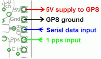
In cases where the location information is not required (modes other than WSPR) or you wish to enter it manually, the serial data input can be left unconnected. The 1 pps input is enough for the frequency lock function. Note that the frequency locking function can only operate in slow-speed modes, or wait periods between messages. GPS lock of the output frequency is indicated by a high signal on connector pin F0.
