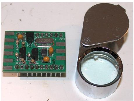
On applying power to the board, you should find a voltage of approximately 3.3V (up to 3.5V) at pin 18 of the module. No output frequencies are generated until you have programmed the Si5351A configuration registers via the I2C interface.
