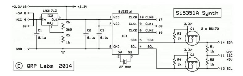
The circuit diagram of the Si5351A synthesizer module kit is shown below.
