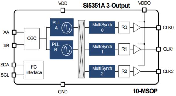
In summary, the Si5351A chip synthesizes output frequencies in three stages. The block diagram of the chip is shown to the above (from the Si5351A datasheet).
