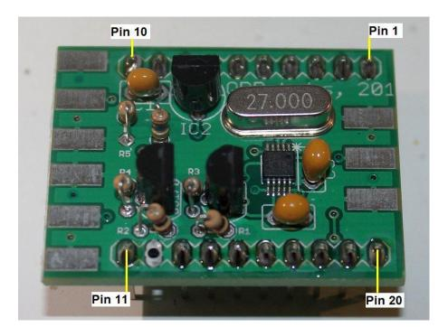
to the physical module, designated pin 1 is near the shorter PCB end of the module, as shown in this photograph.
