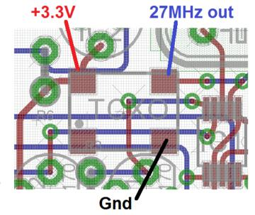
Note that some TCXO's have discrete frequency jumps which can cause problems with narrow-band modes such as WSPR.
