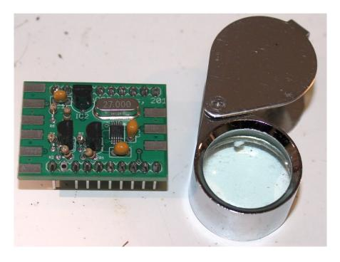
On applying power to the board, you should find a voltage of approximately 3.3V (up to 3.5V) at pin 18 of the module. No output frequencies are generated until you have programmed the Si5351A
